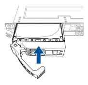
Push the tray lever until it clicks and secures the drive tray in place. The drive tray is correctly placed when its front edge aligns with the bay edge.
