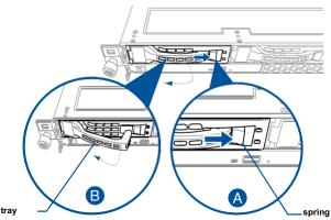
Firmly hold the tray lever and pull the drive tray out of the bay.
