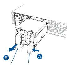
module lever PSU latch
