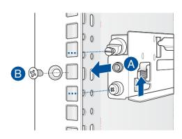
11. Lift the server chassis and insert into the rack rail.
